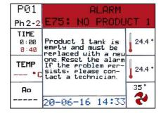
At first the image concerning the alarm is displayed (for 5 seconds); then the alarm description is displayed (for 10 seconds). The image and text alternate until the alarm is reset.
