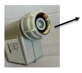
Pull out the cylindrical filter inside the ferrule, cleaning it thoroughly with compressed air if necessary. Place the cylindrical filter in its housing, taking care to insert as photo. Screw the ferrules to the water supply. Open the taps supplying water to the machine and restore the supply.
